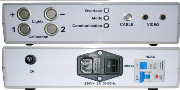
Control module for Dcam with depth sensor
